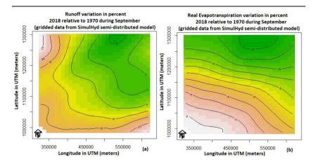
Figure 3: Relative variation of runoff (a) and the relative reduction of real evapotranspiration during September when comparing 2018 to 1970.
